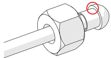
Use grease Molycote G-1502 (COD. 6000000) on the spindles of all copper pipes
