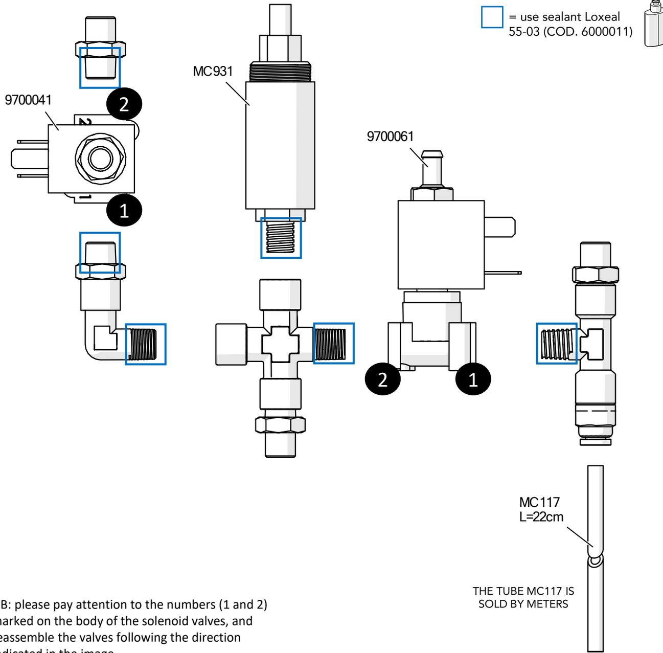
NB: please pay attention to the numbers (1 and 2) marked on the body of the solenoid valves, and reassemble the valves following the direction indicated in the image.
